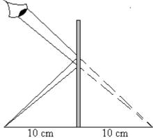
This image is virtual because it cannot be formed on the screen and there is no actual intersection of light rays when the image is formed
