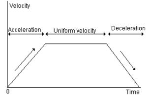
(b) A car moving with a uniform velocity of 100m/s is decelerated at 2.5m/s to a stop. Calculate:(i) The time taken for the car to stop
