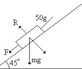
(i) The acceleration of the load as it slides down the slope Given: Mass, m = 55gInclination,  $45^{\circ}$ Weight parallel to slope, mg sin( $45^{\circ}$ )
