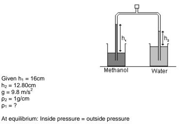
Step 1: Rearrange for ρ<sub>1</sub> Step 3: Solve for relative density Relative Density =  $\frac{Density \ of \ substance}{Density \ of \ water}$  $\rho_1 h_1 = \rho_2 h_2$  $\rho_1 = \frac{\rho_2 h_2}{h_1}$  $RD = \frac{0.8}{1} = 0.8$ Step 2: Solve for p1  $\rho_1 = \frac{1 \times 12.80}{16}$  $\rho_1 = 0.8g / cm^3$
