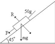
(i) The acceleration of the load as it slides down the slope
