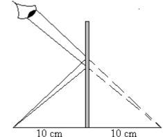
This image is virtual because it cannot be formed on the screen and there is no actual intersection of light rays when the image is formed
